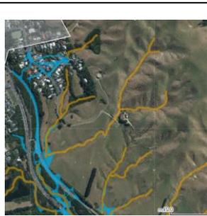
**Figure 7: Flood Hazard Mapping in the Plan indicating modelled stream corridors**
