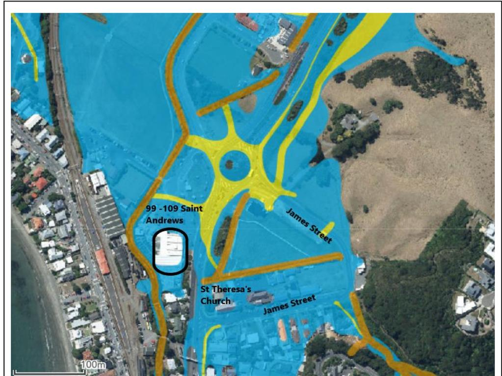
**Figure 13: Flood Hazard Mapping in the Plan indicating modelled stream corridors, overland flowpaths and inundation for 100 year including Climate Change**
