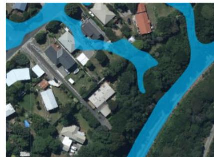
**Figure 4: Inundation Layer for the Flood Mapping showing flooding above 50mm**
