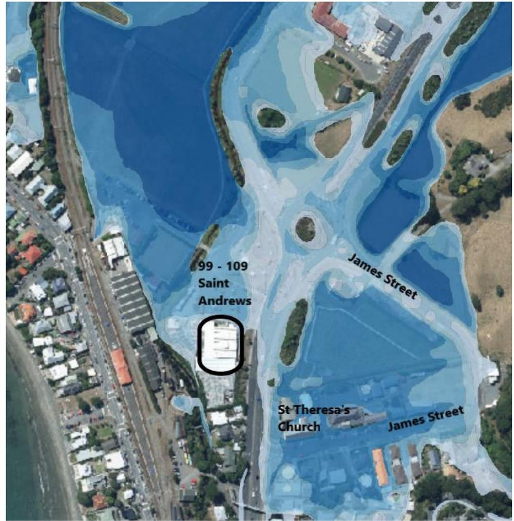
Figure 12: Flood Depth Mapping indicating modelled flood depths for 100-year including Climate Change
